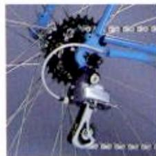
The Edge 14-speed derailleur with indexed shifting allows you to change gears smoothly and accurately.
